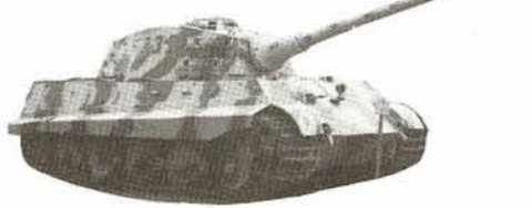
PzKw VIb — the "King Tiger" — armed with a special 8.8cm, KWL 43, L/71.
