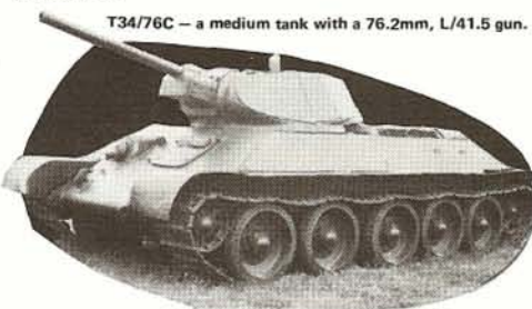
T34/76C — a medium tank with a 76.2mm, L/41.5 gun.
