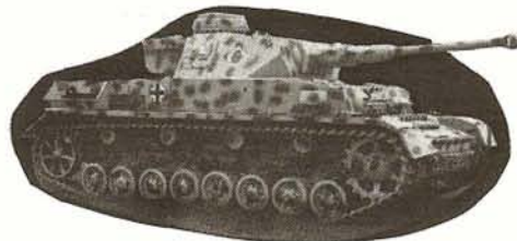
PzKw IV AUSF F2 with 75mm KWK 40. The workhorse of the German Panzer Divisions.
