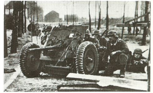
The 3.7 cm PAK was greatly undergunned in comparison to the Soviet heavy tanks they were expected to deal with. The small AT weapons often needed several hits at point blank range to stop an advancing T34. Only the inexperience of Soviet tank crews prevented complete disaster in the early years of the war.
