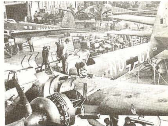
Factory view of He115's and He111's under construction. The two-engined bombers were Germany's largest aircraft and totally unsuitable for strategic bombing. Goering thought otherwise.
