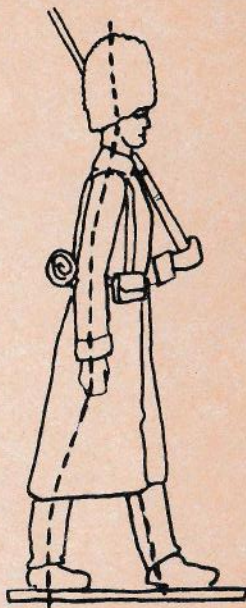
Parting line (dotted line) on a Britain casting of British Guard, overcoat, marching.
