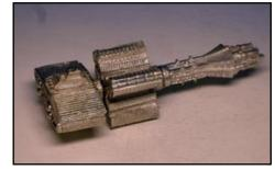
Step 5: Assemble the three parts with pins.
