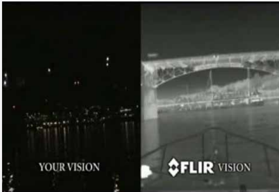
TYPICAL CIVILIAN BLACK & WHITE THERMAL IMAGING DEVICE, USED FOR MARITIME SAFETY (MILITARY DEVICES USUALLY OFFER BETTER CLARITY) NOTE: FLIR - FORWARD LOOKING INFRA RED
