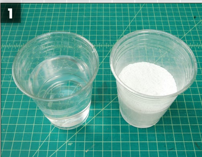
Step 1) Mix your plaster by adding small amounts of plaster into the water, stirring thoroughly each time. You want the consistency to be somewhere around melted ice cream. You don't need to be nearly as precise here as when mixing the silicone.
