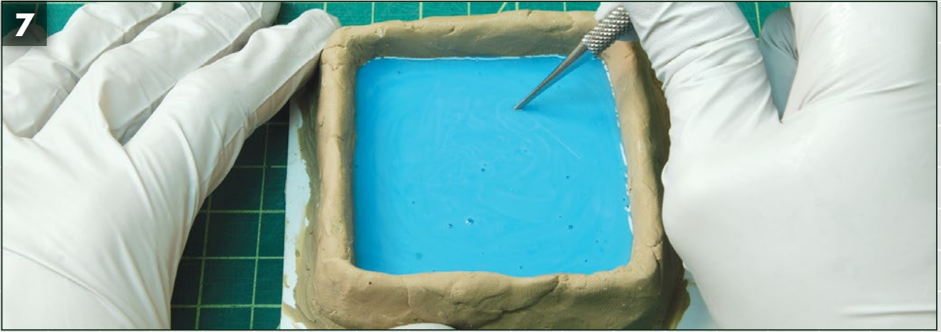
Step 7) Use a needle tool to gently poke all the corners to release any trapped air.
