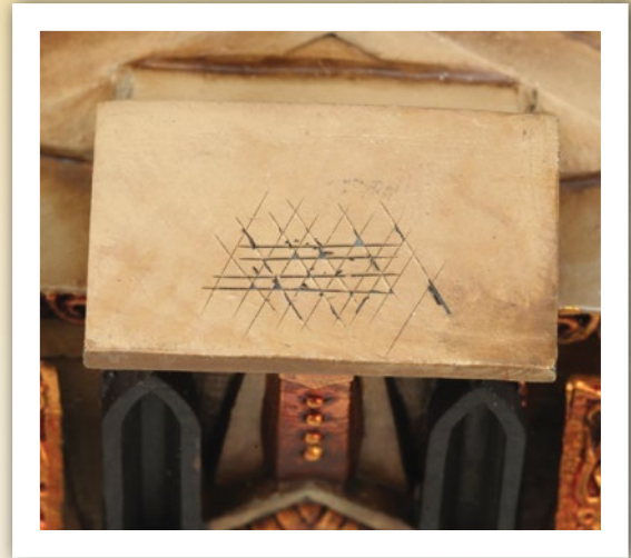
Gluing adheres poorly to paint, so when gluing painted surfaces score the surface with a hobby knife. This gives the glue some rough spots to seep into.
