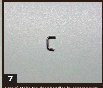
Step 7) Make the door handles by shaping wire into a U shape.
