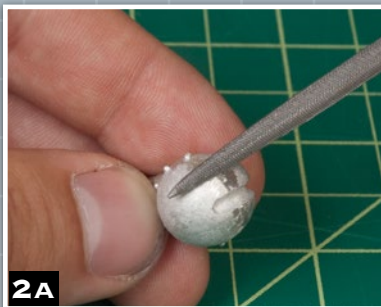
2A Filing/Sanding: Next, use your Formula P3 File Set and fine grit (150–350 grit) sandpaper to thoroughly clean the parts. Remove any mold lines and erase all signs of mold shift. You can also take time at this stage to sharpen the spikes and axe for a more realistic look.
