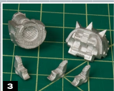
3 Scouring: This lesser-known technique reinforces smooth joints between parts and can be far more effective than pinning. To scour, use the tip of your hobby knife to gouge a crosshatched pattern into the surface to be joined. This effectively doubles or triples the surface area being bonded and creates a joint so strong that parts will bend before they break apart. The Extreme Juggernaut's massive size means that even the finger joints have enough surface area to be effectively scoured and thus do not require tedious pinning.
