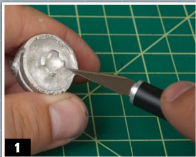
1 Trimming: In any modeling project, you will first use a Formula P3 hobby knife to trim away any flash and venting left over from the casting process.
