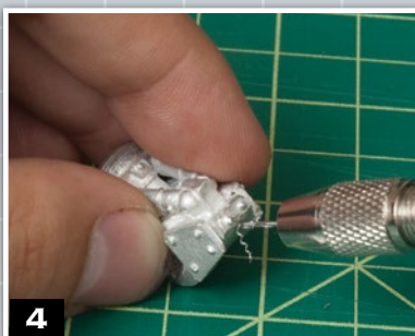
4 Pinning: Even though the vast majority of the Extreme Juggernaut can and should be scoured, three sections do require reinforcement with pins. To avoid drilling into a partially assembled model, drill the holes before assembly using a .85 drill from the Formula P3 pinning set. The hip joints and ankle both need to be carefully pinned, as the weight of the upper body can exert quite a bit of pressure on these joints. Because the contact area on the front and rear mud flaps is so small, pins ensure these pieces stay joined. Scour to strengthen all these joints further and create a rock-solid model.
