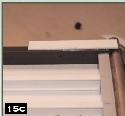
Step 15) Add support for the hinge mechanism. Add small angle bracing along the bed of the bridge to mast the join with the large I-beam. Use super glue to adhere the large gears to a large piece of brass tube. Affix the assembly to the rear of the bridge. Use plastic glue to attach a piece of plastic card to the bottom of the large I-beam under each gear. Use super glue to adhere the gear to the plasticard piece.
