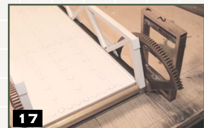
Step 17) Add the gear towers. Next, you will solder two gear towers to the brass tube you just assembled. This can be a very difficult step, because the gears on the bridge must line up with a small gear on the top shaft. The bottom shaft must also clear the tube or the far gear tower will not work. You should trial-fit the pieces before you solder the joint.
