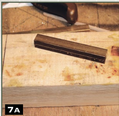
Step 7) Align and drill the box tubes. Cover two opposite sides of the box tube with black marker and draw a line down the center of the piece. Using a power drill, you will need to drill a hole on each side of the box tube. Make sure the holes line up with each other exactly, then drill one hole at a time. Do not try to drill all the way through from one side to the other, as the holes will not line up properly.
