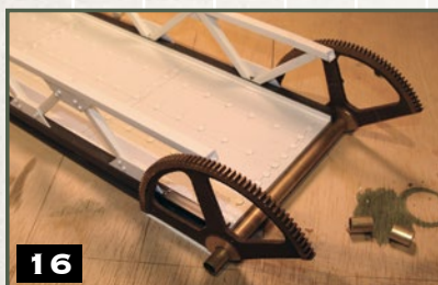
Step 16) Solder the tubing leading to the gear assembly. Insert a brass tube into the gear assembly. It should fit just inside it. About 1/2" should stick out on each side. Cut two pieces of the larger brass tube. Carefully solder the larger pieces onto the smaller tube. Do not let the solder touch the gear assembly or the bridge will not work.
