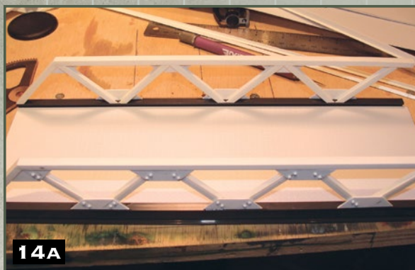
Step 14) Add braces and supports. Cut a piece of diamond plate plastic card and glue it onto the surface of the bridge. Turn the bridge over and glue small I-beams between each square box tube.
