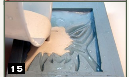
15 Step 15.) For this next step, mix up some Plaster of Paris (although you can use resin). Before pouring the plaster, mix some water and Jet Dry® in a spray bottle and mist the mold with it—this helps prevent air bubbles occurring. Gentle tapping of the mold also helps remove excess air bubbles.
