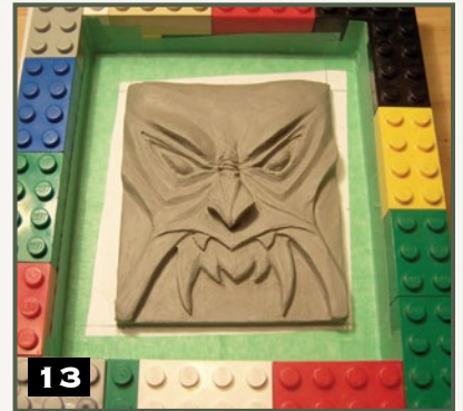
13 Step 13.) After shaping everything with the clay, create a square around the sculpture using connecting blocks. Once the blocks are in place, it is very important that you seal them with painters tape. The two-part silicone rubber mold material will seep through the small seams in the blocks and sealing the blocks with tape prevents this. Mix the silicone following the instructions. When applying the silicone to the sculpture, drizzle it on in a thin, almost transparent layer. If you just pour the mixture in, you run a high risk of having air bubbles attach to your sculpture, thus ruining your mold.
