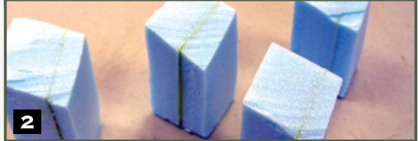
Step 2.) Take the hot wire cutter and make a 45-degree angle cut along one end.
