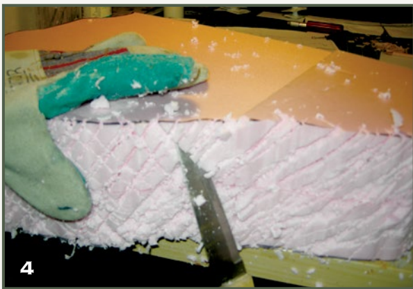
Step 4.) Now it's time to cut out your tunnels. A foam cutter works best, but if you do not have access to one, a keyhole saw or hack saw blade works just as well. The last two tools will scar up the foam, but you want this—the foam is supposed to look like rough rock face. Always use safety goggles and leather gloves when cutting foam. Then, using a heavy blade make diagonal cuts at various depths, followed by more cuts at the opposite angle.
