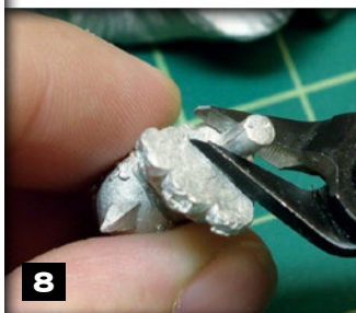
Steps 7 & 8) Clippers make the best tool for removing bits from their metal sprue, such as the Rhinodon's spikes and the tab on its right foot. Keep the flat side of the clipper blades against the part for a flush cut. Take care, since the clipped pieces tend to go flying. Holding your finger over the part or angling the piece toward the desk keeps the part from shooting across the room. Wearing safety approved eye protection is the best way to avoid serious injury.
