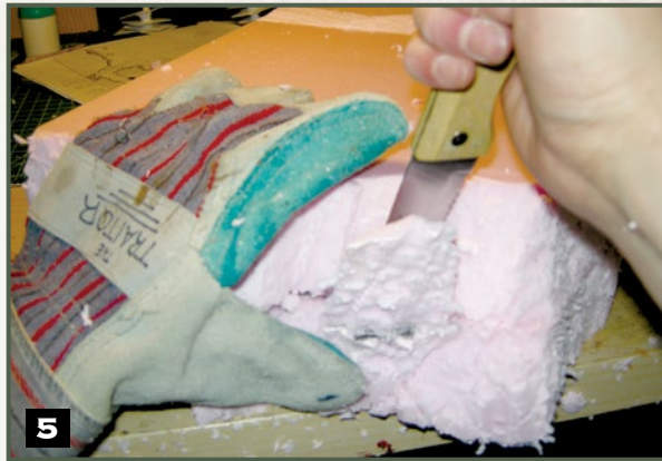
Step 5.) Once you have a crisscross pattern, get a very sturdy, thick knife with a serrated edge, such as an old bread knife. Drag the serrated side of your knife across the foam. If you were using a keyhole saw, this is where you will start using your knife. Starting at the top, plunge the knife in the rock and pry out the foam. Continue until you have the desired effect.
