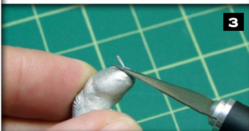
Step 2 & 3.) Flash is the excess metal that squeezes out from between the two halves of the mold during casting. Carefully slice around the edge of the piece with the hobby knife to remove this excess metal. You can go back and smooth the edges with a file later.
