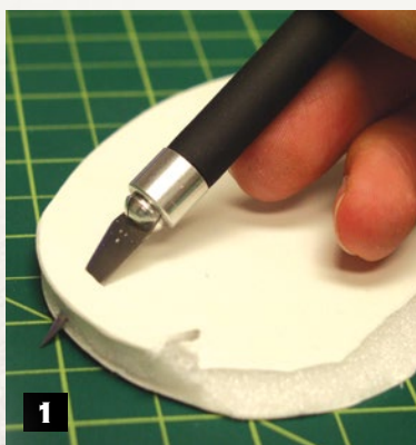
1 Step 1.) Start by cutting some 4" - 6" diameter circles out of 1/4" thick foamcore as the bases for the craters. Bevel the edge of each one with your hobby knife.
