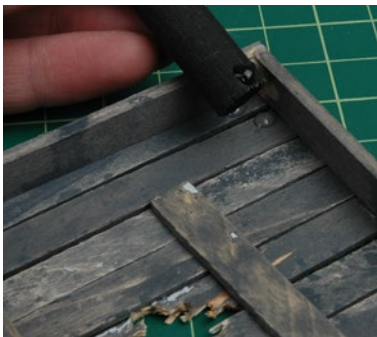
After the paint dries, glue the pylons to the frame. For this I used superglue and accelerator. I placed one drop on the pylon and one the plank.
