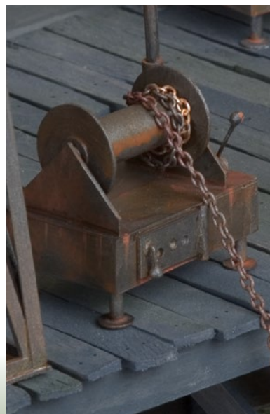
Steam Winch assembled and painted
