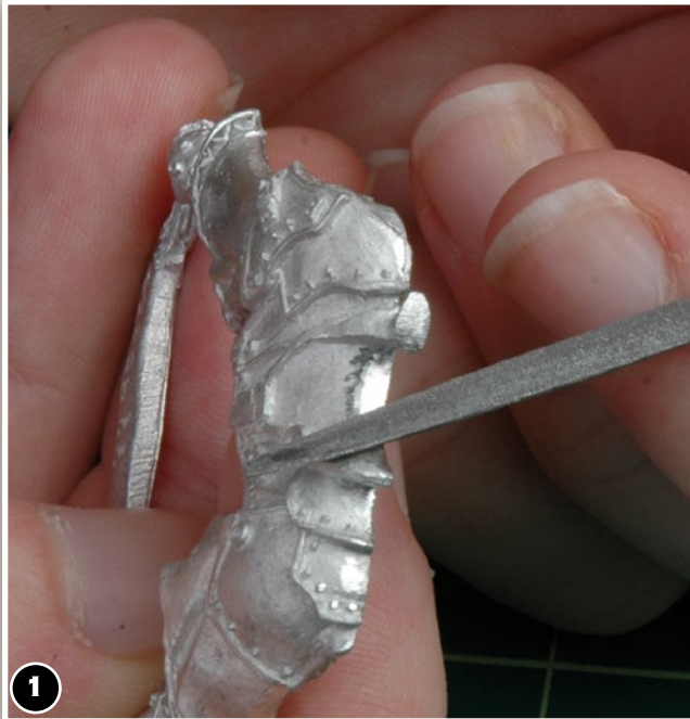
1 Use a needle file to carefully smooth away any mold lines.
