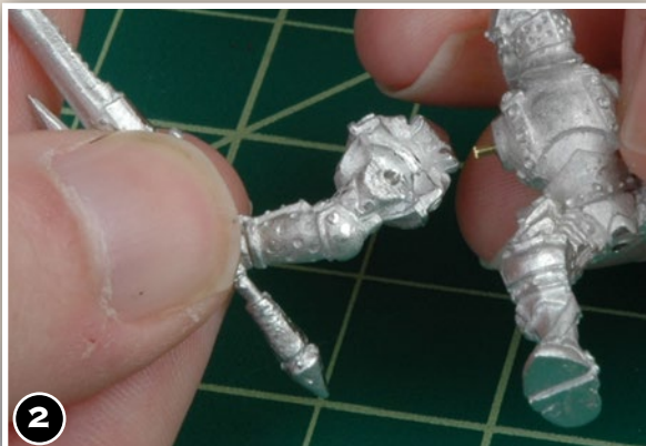
2 A short strengthening pin really helps to keep lance arms from breaking off when you are playing with, or transporting, figures.
