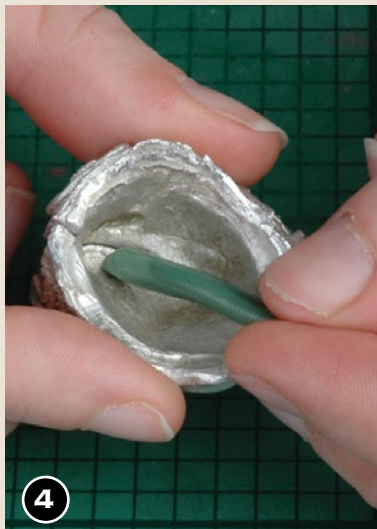
4. One extra step to ensure that the legs are solidly joined together is adding some putty to the inside of the join. Roll out the putty into a thick sausage and press it along the join.
