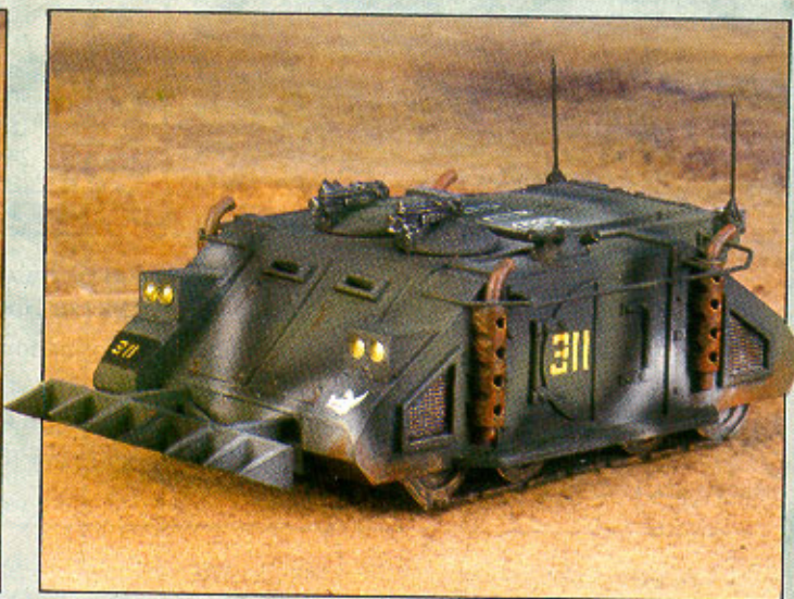
An early Rhino kit experiment by Sid. Note the headlamp cavities. They were painted yellow and filled with PVA glue. The glue becomes transparent when dry, hence the realistic headlamp effect.
