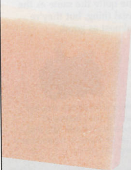
Chad used pink insulation foam – available from most DIY stores – but polystyrene would work too.
