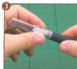
3 Replace the sheath and screw the blade mount back onto the handle.
