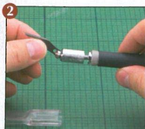
2 Replace the old blade with a new one, taking extra care when handling naked blades.
