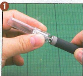
1 With the sheath on, unscrew the blade mount from the knife handle.
