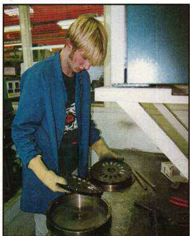
Metal studs are placed around the circumference of the mould so that the two halves can be located together easily and accurately every time.
