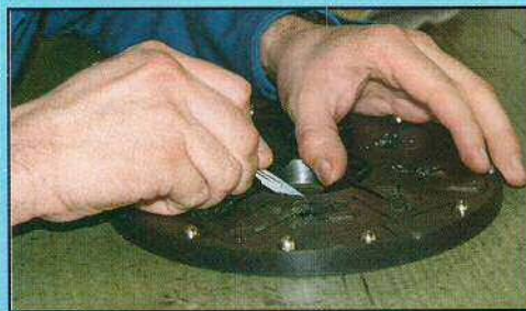
Cutting in channels for molten metal to flow in and air to flow out.
