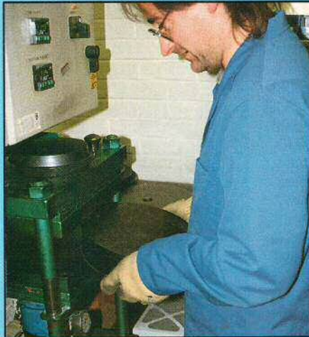
Placing the master mould in the press.
