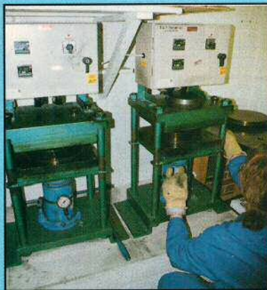
A master mould is pressed into shape.
