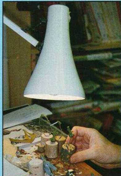
Placing the masters under a hot lamp helps them to harden faster.
