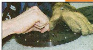
The pressure of the mould making machinery must be careful monitored. Too little and all the detail will not be picked out, too much and the mould will be distorted.
