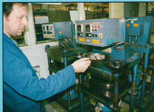
The "tins" are left to warm up for five minutes, before being carefully arranged on the rubber.
