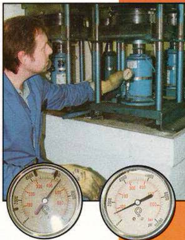
The pressure of the mould making machinery must be careful monitored. Too little and all the detail will not be picked out, too much and the mould will be distorted.
