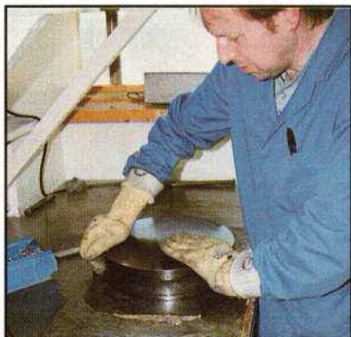
Metal studs are placed around the circumference of the mould so that the two halves can be located together easily and accurately every time.
