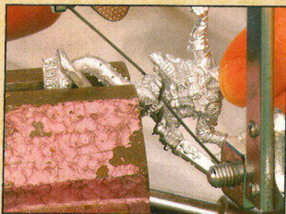
The miniature is held in a vice by the tail section and the upper body is carefully removed with a fret saw.
