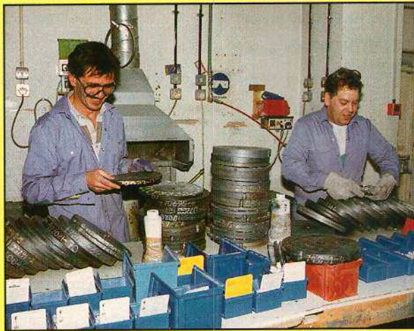
A set of miniatures is cast up in the Citadel foundry.
