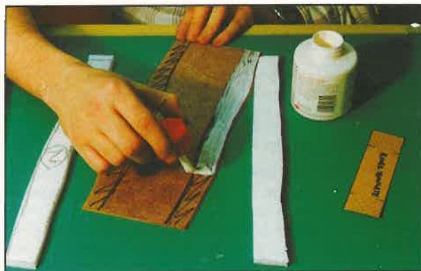
Gluing the banks to the baseboard.
