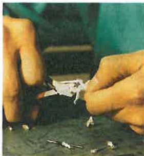
Photo 2: The original head is removed with a pair of cutters
