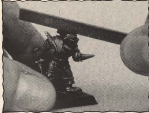
A file is used to begin the flattening process.
