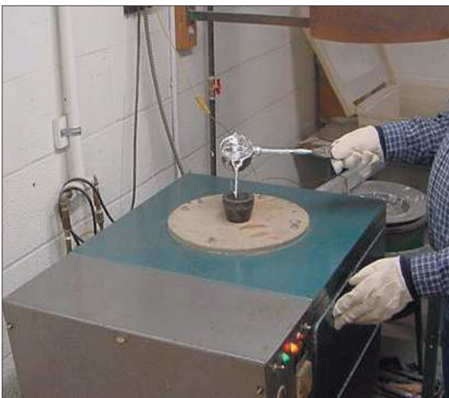
STEP 5 -Pour melt pewter while spinning..
