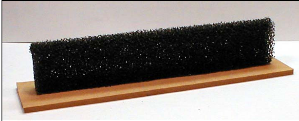
Image 3: Filter foam glued onto the MDF base.
