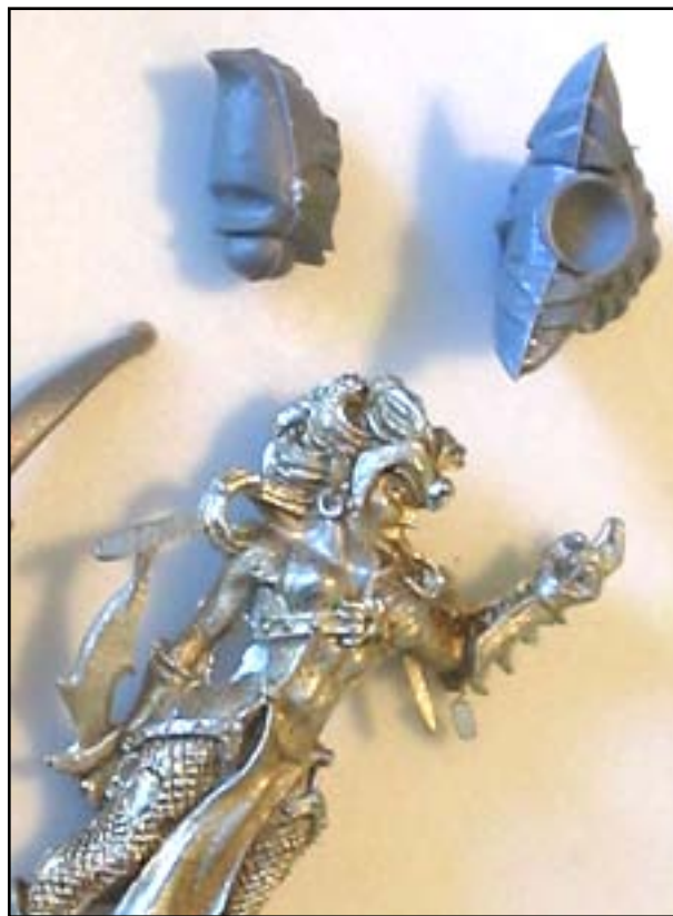
Examples of common casting defects. Mold lines are visible on the helmet and breastplate. The tip of the Drannach has a small disk of flashing. The Witch Elf has several sprue tags. Each of these will be easy to remove, but is important to the quality of the finished pieces.
