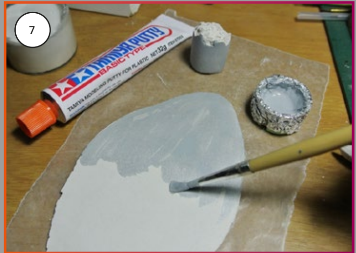
7. After it has dried, the surface was not smooth enough and had some little wavy areas. I solved this problem with Tamiya putty diluted with thinner and painted over the whole sheet as well as the columns, then sanded with 400 and 600 grit sandpaper.
