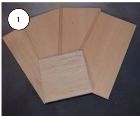
1. First, I cut the 5mm thick balsa wood into four 20cm long and one 10,5 cm long strips. The four would be my walls and the shorter 10,5 x 10,5 cm will serve as the floor of the roof.
