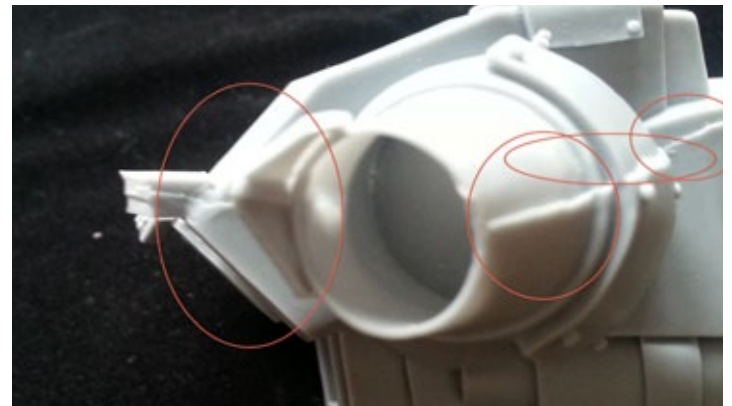
Detailed flash lines and blocks on the back of the exhaust of the body.
