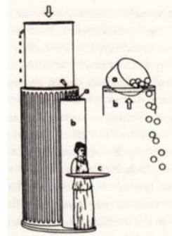
Figure 7: Plato's Water Alarm Clock [6]
