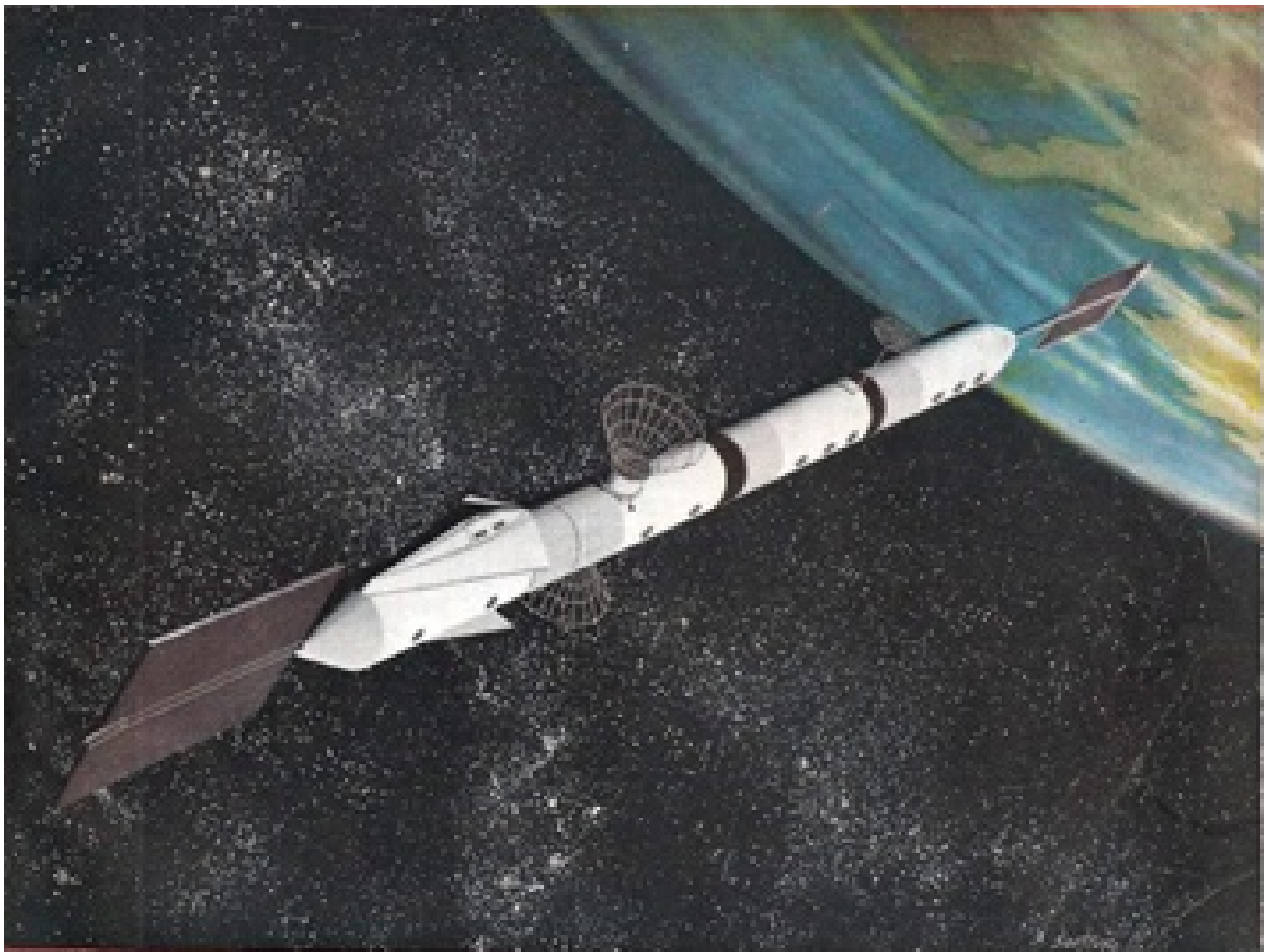
Station I above Earth. Stations II and II built to same plan. A re-entry vehicle (Hermes 3rd stage) is docked to the top front, while the round “cage” is for entry to the station after a short spacewalk.
