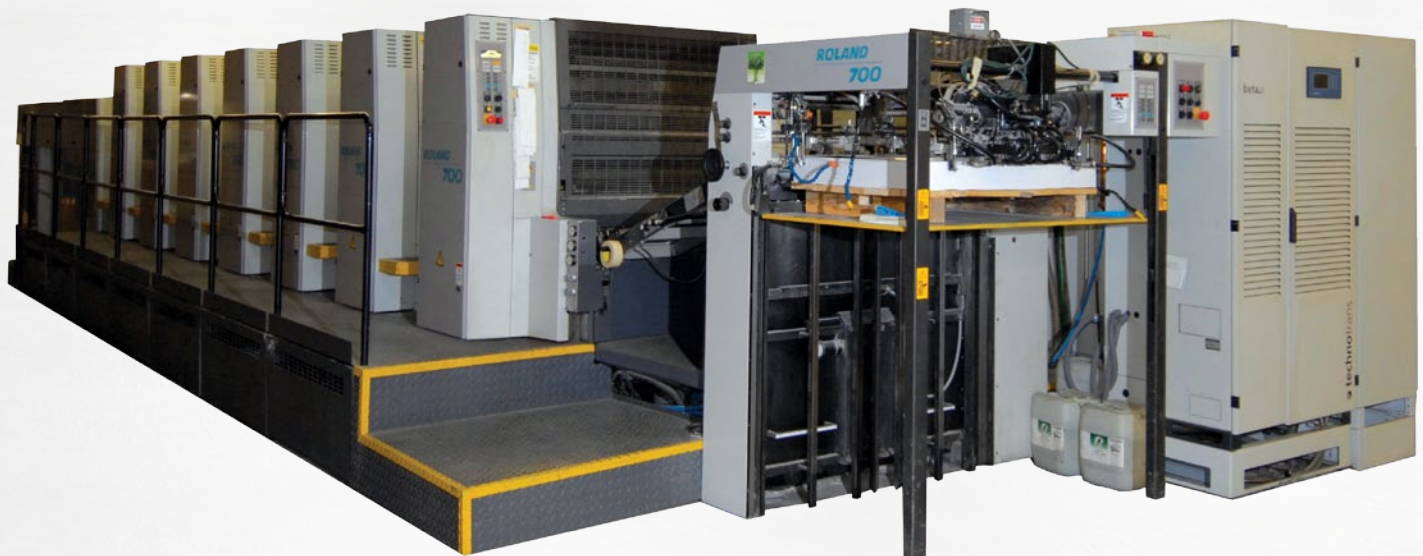
Man Roland 700 series press (6 color with inline coating)
