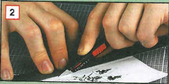
2 Turn around the banner leaving a border all round of about 2.5cm.
