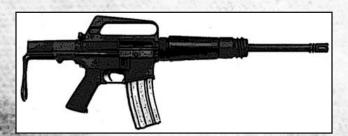
To enter the submachine gun market, Colt modified the M16 platform from a gas-operated rifle in 5.56x45mm NATO to a blowback-operated 9mm submachine gun. The upper is based on that of the M16A1 but has a 10.5"-long barrel. The lower's magazine well features an adaptor to allow the use of modified Uzi submachine gun magazines. Both of these models have a 10.5" barrel. The RO635 is fully automatic, whereas the RO639 is limited to threeround bursts.
