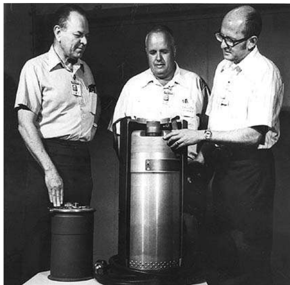
Above: The code-decoder/firing unit (left) and the packing container for the MADM. The entire unit weighs about 400lbs (181 kg.).
