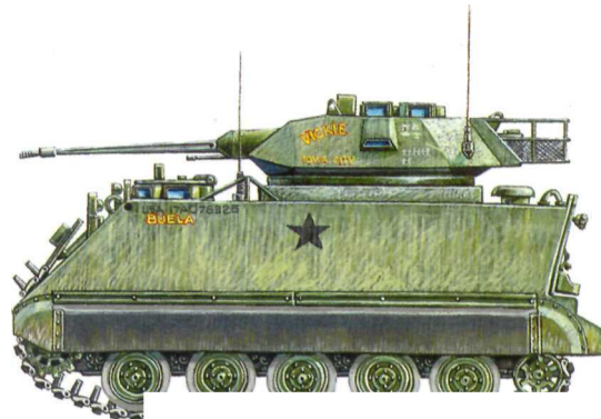
E4: M115A1 armored cavalry combat vehicle of 163rd Armored Cavalry Regiment (Montana National Guard); Korea, 1998.
