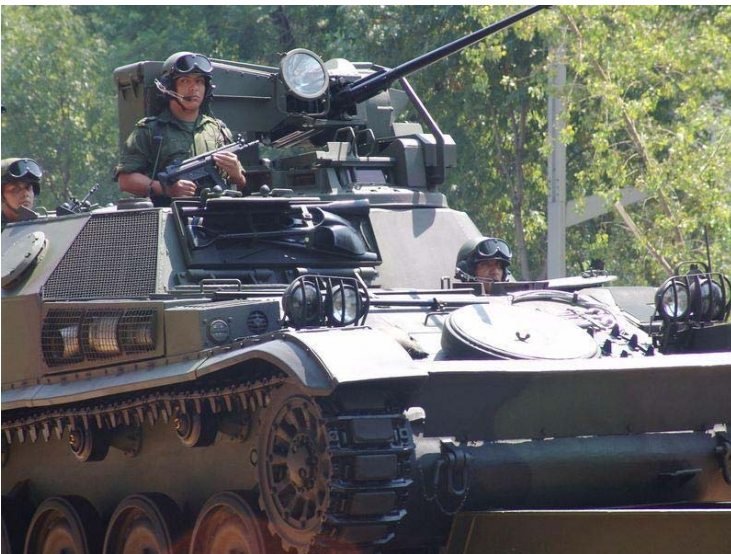
Mexican Armored infantry crewing a refurbished AMX-VCI Toucan equipped with a 20mm GIAT auto cannon.
