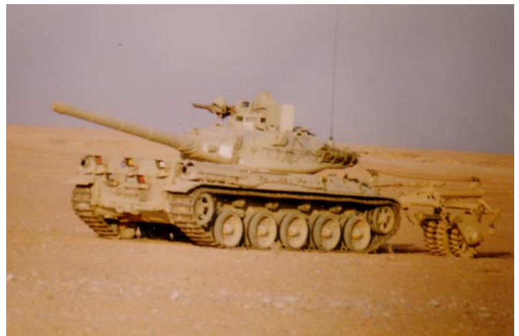
An AMX-30S which has been converted to an engineering role.
