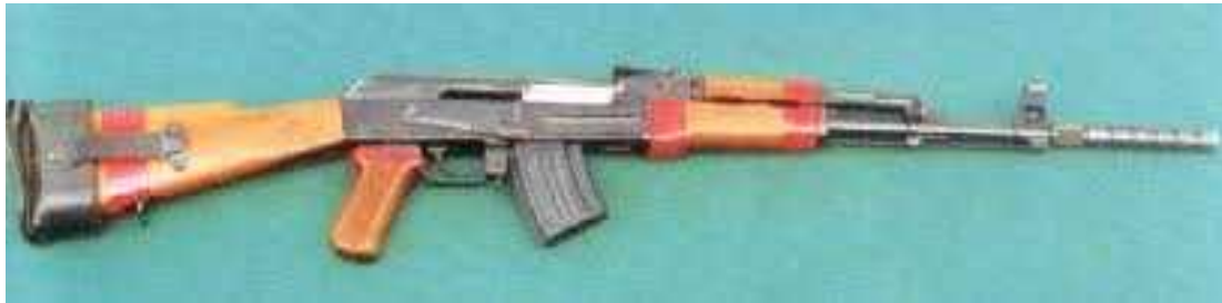
Illustration 29: Kbkz Wz1960 showing butt padding and special 10 round magazine. Note the slightly different muzzle compared to the Yugoslavian version. Warsaw Collection.
