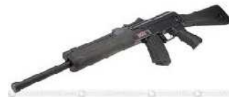
Illustration 17: A locally crafted AK in .410 shotgun note the all new front end. (Ukrainian Military Museum)
