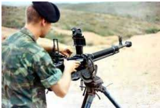
Illustration 89: US Ranger test firing a DShKM using the wheeled carriage in it's anti-aircraft mode although without the AA sights. Ranger Regiment Museum
