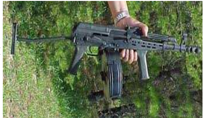
Illustration 18: AMD65 fitted with a 75 round RPK drum (National Geographic)
