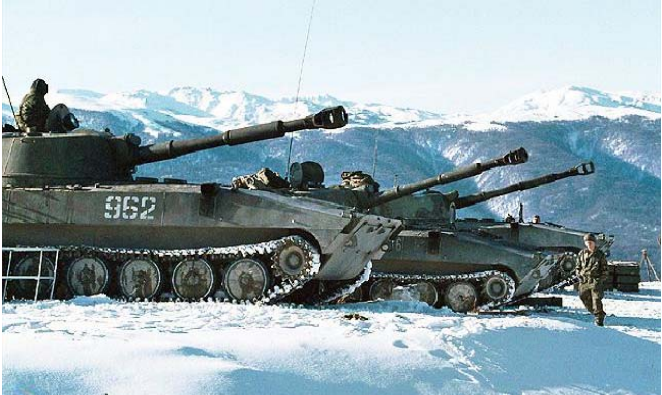
SAU-122/2S1 self-propelled howitzers of the 1 st Tank Division preparing to deliver supporting fires for a Warsaw Pact spoiling attack into Bavaria, January 1997.
