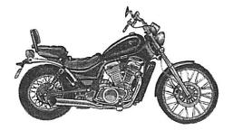
The only real difference between the three Intruders is in their engine sizes, as they all look the same and are almost the same size. It is difficult to tell them apart from a distance. Each has a water-cooled V2 engine with a five-speed transmission, and a single disc brake on each wheel.
