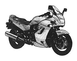
A heavy sports bike, the GPZ 1100 has very high performance despite its somewhat high weight. As most similar bikes, there is room for two people on the buddy seat, the passenger having a small handhold behind the seat. A streamlined cowling is installed over the headlight and engine to reduce air resistance, and a small windscreen helps streamline the rider as well.
