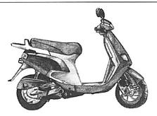
Known generally as "Vespas," these two simple, lightweight scooters are both very similar. Each has a single-cylinder, 125 cc engine and an automatic transmission, so performance is limited, but comfort when riding is high. Two people are seated easily on the buddy seat, with the bike's front plate shielding the driver's legs. There is a small storage space in the front shield, large enough for a small bag, for example.
