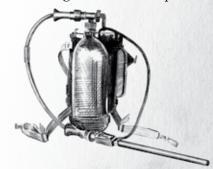
**Type 93:** Issued three years ago, the Type 93 portable flamethrower features three cylinders containing 3.25 gallons of fuel. It weighs only 55 lb., has a range of 25 feet, and a fire duration of 12 seconds.
