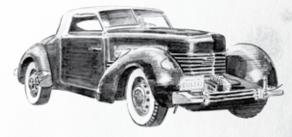
**DeSoto Custom Six Airstream:** Streamlined and affordable. With individual front wheel springing, DeSoto Ride Stabilizer, and hydraulic shock absorbers adjustable to load and road conditions, the new Airstream promises a smooth, comfortable ride. \$700
