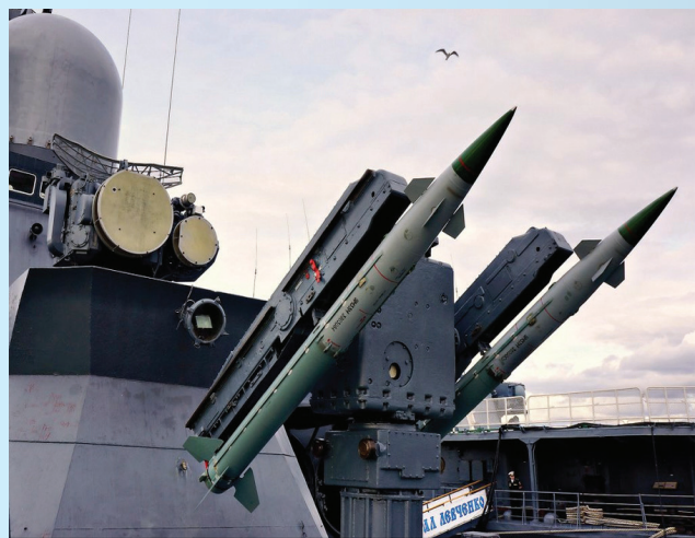
ZIF-122 twin launcher for OSA-M [SA-N-4 Gecko] surface-to-air missiles (bastion-karpenko.ru)
