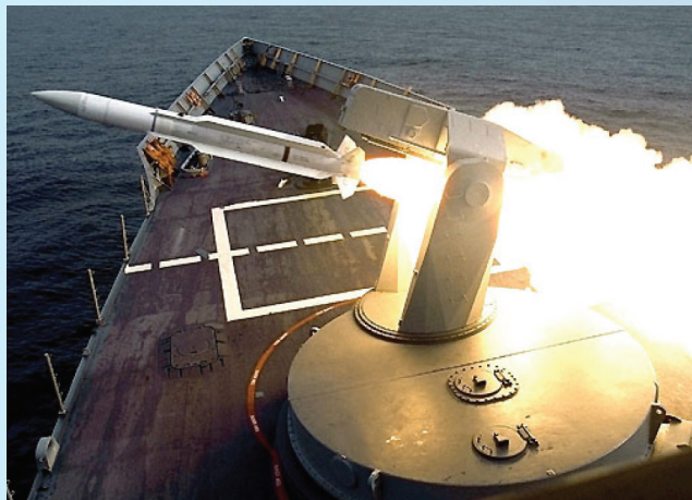
Mk 13 launcher firing a SM1MR missile. (US Navy)
