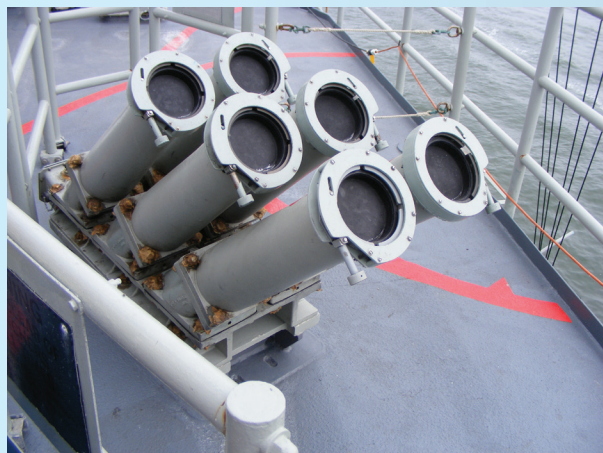
Mk 137 Super Rapid Blooming Offboard Countermeasures (SRBOC) chaff launcher (US Navy)
