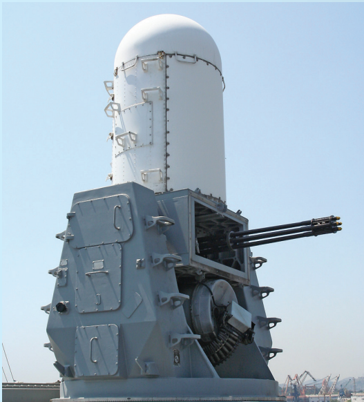
Mk 15 Phalanx Close-in Weapon System (US Navy)
