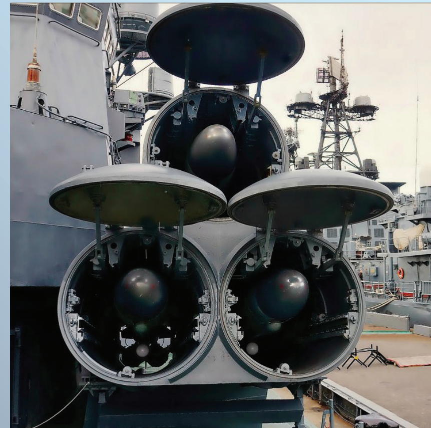
KT-120 triple cell launcher for P-120 Malakhit missiles (wiki.wargaming.net)
