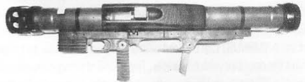
Armbrust with stocks and sight extended for firing
