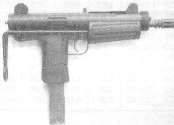
Viking with stock folded and bolt in forward position
