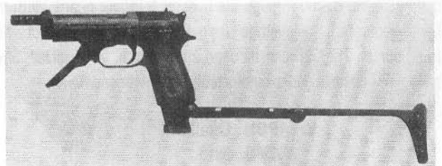
Beretta 93R with stock attached and extended
