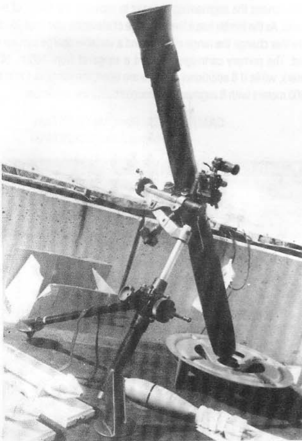
81mm L16 Mortar setup for firing
