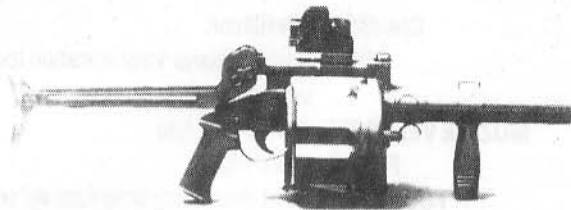
ARMSCOR 6 rd 40mm with buttstock extended and sight set to 0
