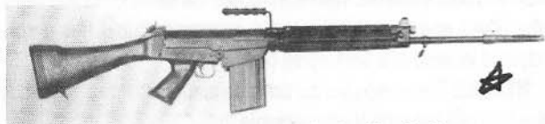
FN FAL with folding carrying handle raised
