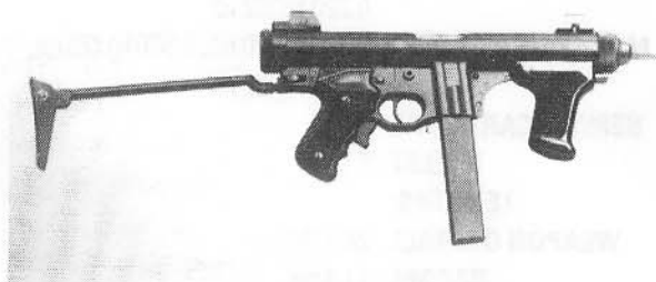
PM-12S with stock extended and bolt forward
