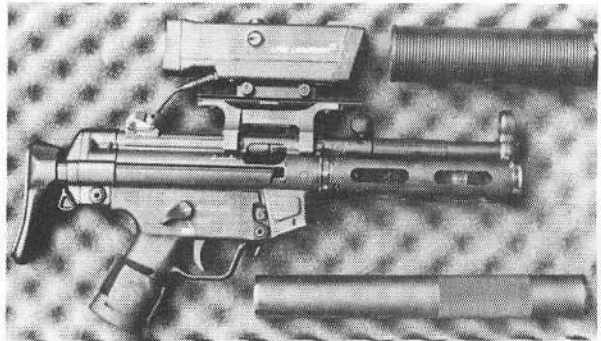
MP5 SD3 with buttstock folded, twin (stacked) 30 rd magazines, and telescopic sight on a quick removal mount
