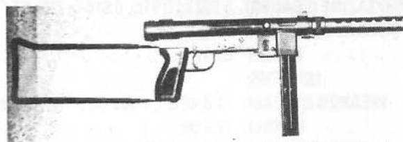
Smith & Wesson M76 with stock extended, bolt forward in the fired position and selector set to safe
