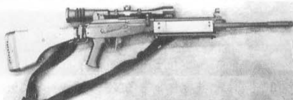
Galil Sniper without magazine, bipod is folded and selector set to safe
